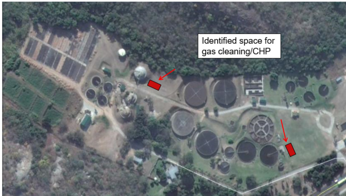
Figure 2: Proposed location of the CHP plant
