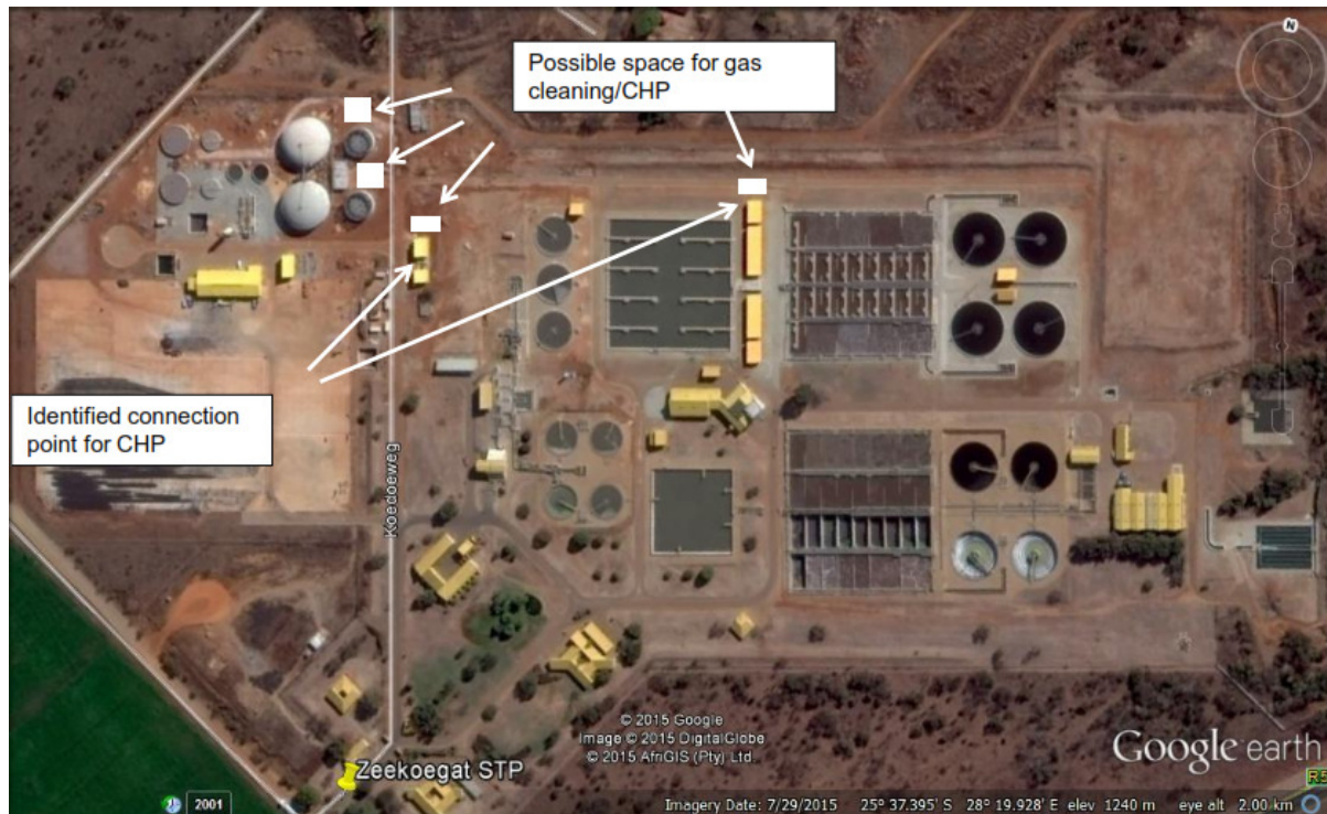
Figure 2: Proposed location of the CHP plant
